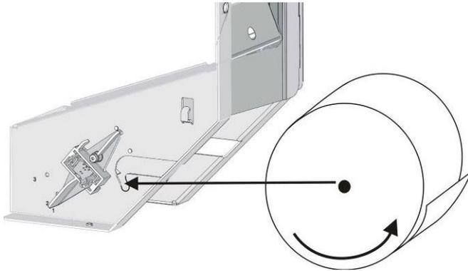
Insert the black mark sensor (top left, top right, bottom left, bottom right) when using paper with black marks.
