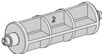
Holder for 25 mm core diameter (identifier 2)
