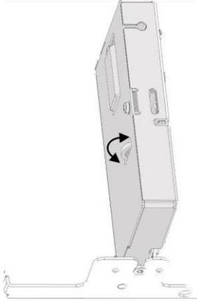
Check the print area of the thermal head for paper scraps. Use the green lever and flap the printing unit upwards.
