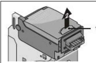
Pull release lever (1) of the validator unit upwards and raise the upper part of the validator unit (2) to the rear.
