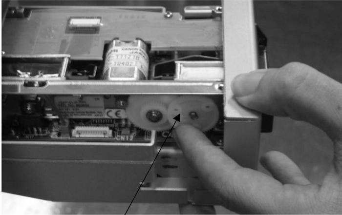
Rotate roller in anti-clockwise direction
