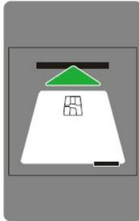
Insert the ID card into the card reader. The card will be motor driven & transported into the card reader.
