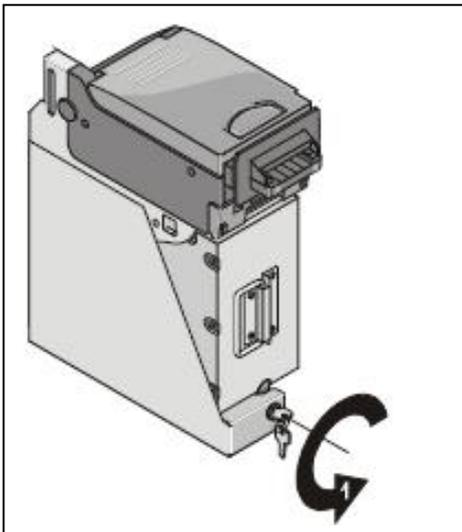
Insert the key in the lock (1) and turn it as far as possible in the direction of the arrow (1) and pull out the key from the lock.
