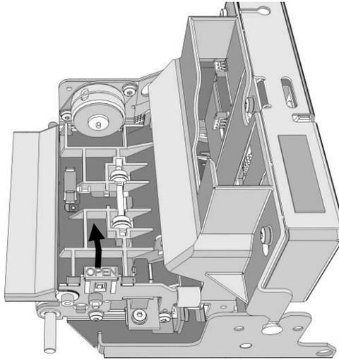
Check the paper transport path and remove the paper scraps, if necessary.
