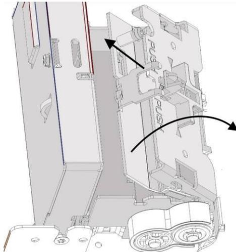
Cut off the remaining paper at the paper support and pull it out.
