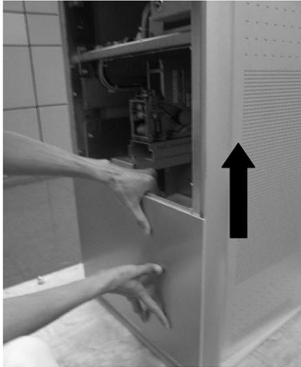
**Inserting bottom front panel:**
