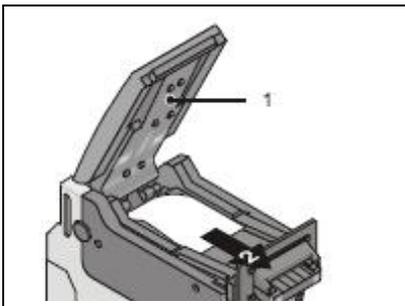
Hold the upper part of the validator unit (1) in the position shown here and remove any jammed banknotes in the direction of the arrow (2).
