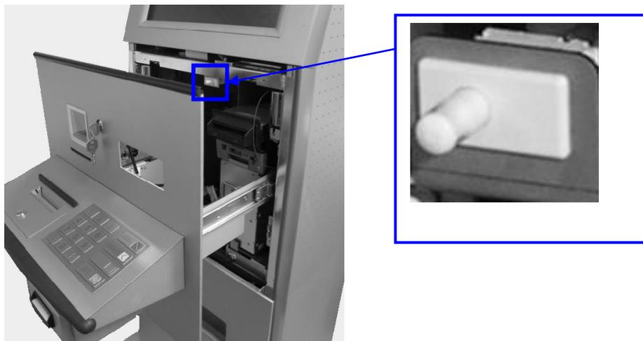
The door sensor is located at the chassis frame underneath the display (see picture above).
