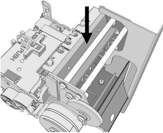
Take the front edge of the paper over the upper axle and feed it into the paper support (see arrow).
